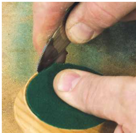
▲ Pic.35 Use the back of a blunt knife to push the baize into the groove. Take your time doing this and it will end up really neat, much better than just sticking it onto the bottom
